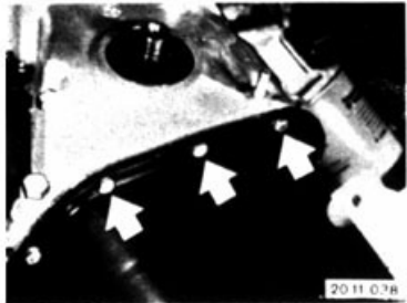
Unscrew front oil pan bolts. Loosen all other oil pan bolts.
